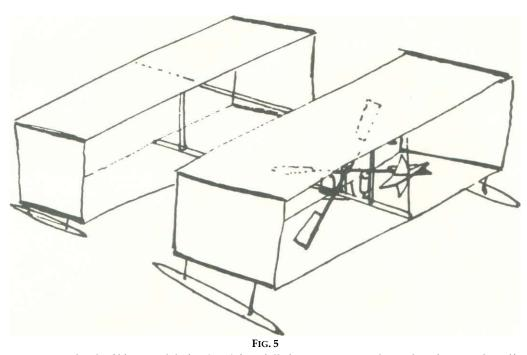
Hargrave's sketch of his second design (1896) for a full-size power operated aeroplane for operation off the water. The machine was not built, as four engines designed to power it were all failures
