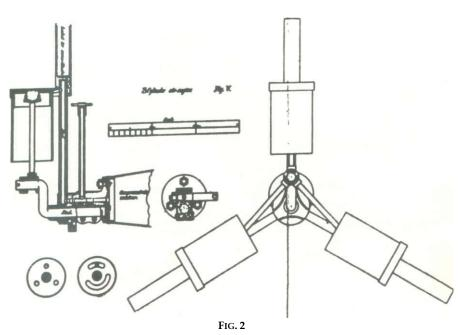
Hargrave's drawing of the three cylinder radial rotary compressed air engine invented 1889
