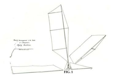
Hargrave's perspective drawing of india rubber powered flapper operated flying machine of 1885
