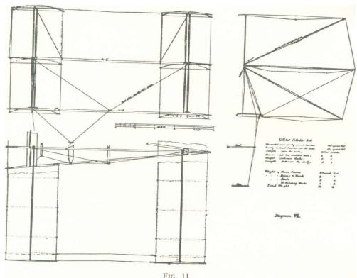
Hargrave's drawing of his 158 sq. ft. triplane box kite of only 25 lb. weight of 1895 showing the development m the design of supporting surfaces culminating in the 1902 aeroplane
